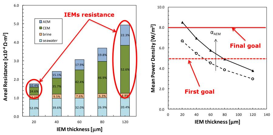
Simulation of a 1000 cells stack assuming a linear decreasing of IEMs resistance with IEMs thickness.  $\alpha_{AEM} = 0.65$ ,  $\alpha_{CEM} = 0.90$ . Spacer thickness of seawater/brine compartments  $\delta = 200 \ \mu m$ .
