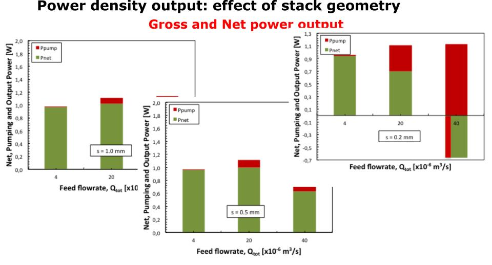
Simulation of a **50-cells stack** with **200**  $\mu$ **m** spacers; rectangular distributor/collector with thickness s= 0.2 - 0.5 - 1.0 mm; external load is assumed equal to stack resistance
